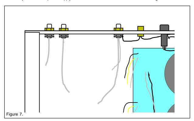
Use the black screws to secure the power supply board. Feed them from the bottom of the chassis and into the plastic standoffs on the bottom of the circuit board.
