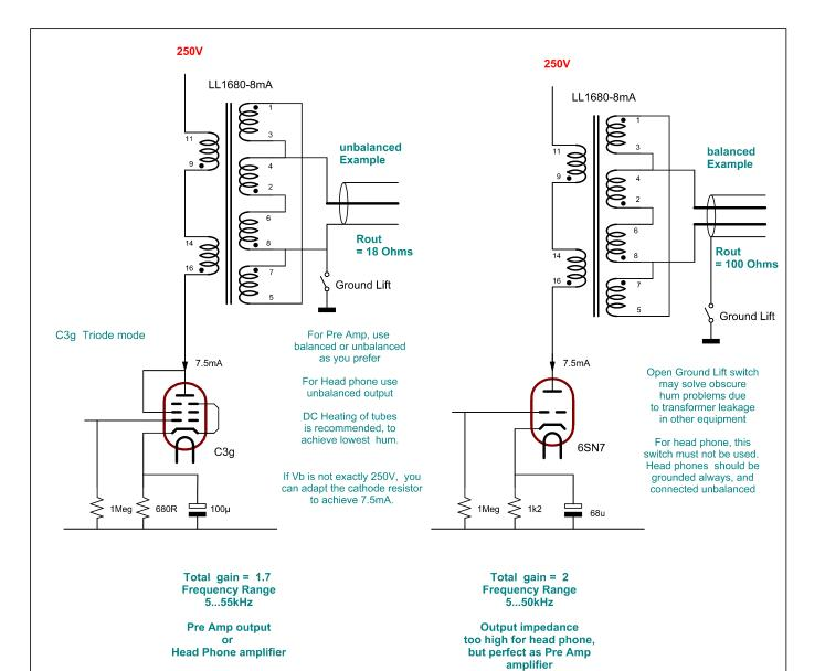
We show here some applications of the Lundahl LL1690 transformer. It was made to meet or exceed the specifications of the legendary UTC transformer LS-27. This transformer, originally used by RCA in Tube Mike Preamps, such as the famous BC-2B Console is still am expensive item.
